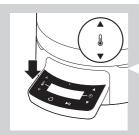
2 Press the temperature increase or decrease button one or more times to set the required temperature.
